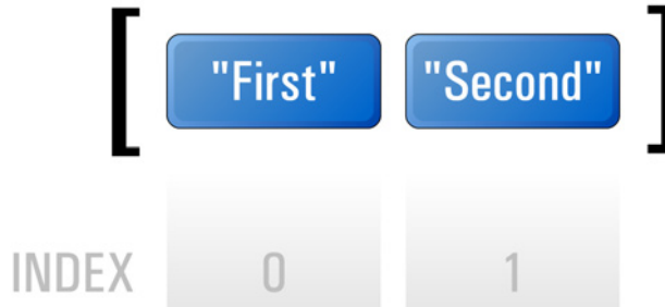
Figure 2.4. An array storing data sequentially, with an index for each element, starting at 0
